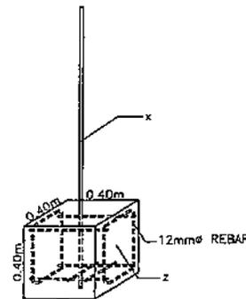
**ANCHOR BLOCK WITH REBAR**
